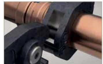
8. Engage the actuator and check insertion depth
