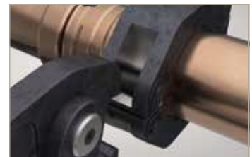
8. Engage the actuator and check insertion depth
