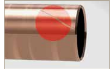
4. Check for scratches & scores
