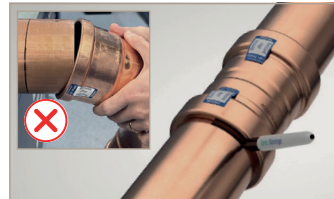
6. Mark the insertion depth
